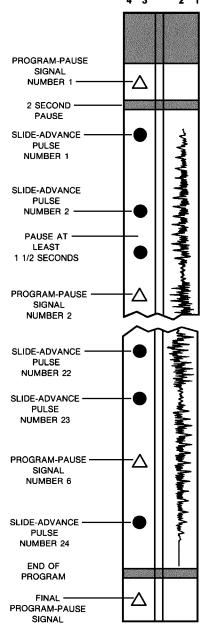
Hz slide-advance pulses and 150 Hz program-pause signals. Like most cassette machines designed for audiovisual use, the tape is intended for recording and playing in one direction only and must be rewound before being replayed.
